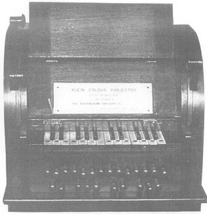
Fig. 6. The two-octave controller of Adrian Klein's color projector for stage lighting (1920). This instrument demonstrated Klein's color theories in which the visible spectrum was logarithmically divided.
